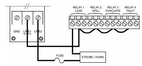
Jumper the 'Neutral' line of an external power source or the monitor's AC input to the 'Common' terminals on the relay connector.
